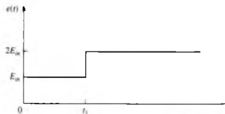
Figure 10-12 Input voltage waveform for the network in Fig. 10-3.
