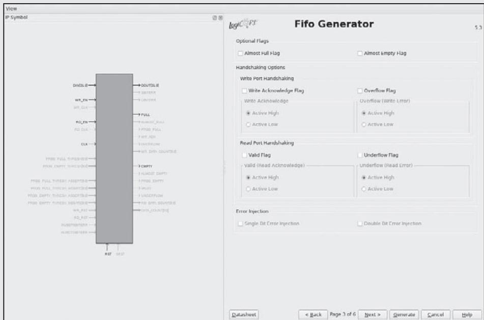
Figure 2.33. CoreGen's FIFO Generator handshaking signals page.
