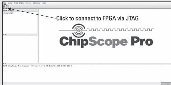
**Figure 5.23.** Xilinx ChipScope Analyzer Pro main GUI with “Open Cable” button identified.
